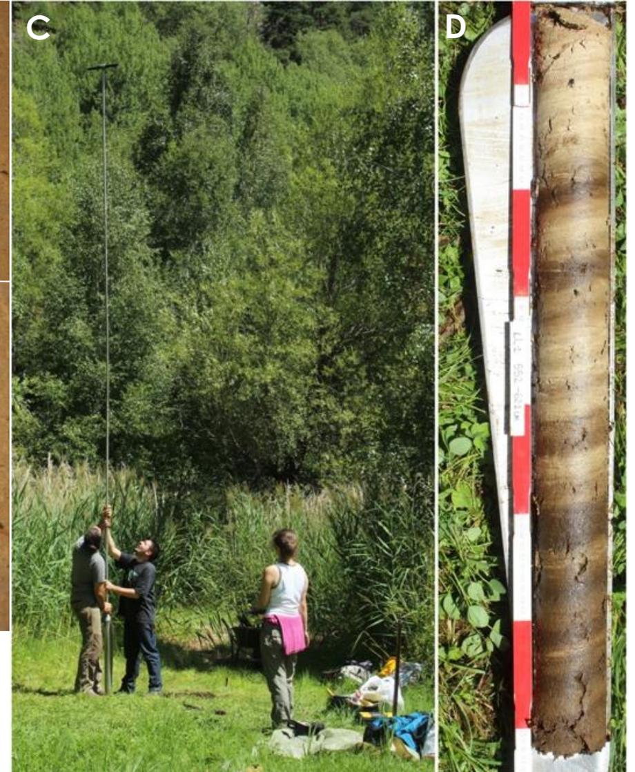
A) and B) Undisturbed peat and lake sediments corers (russian corer); C) coring through the deposits of the Lolair lake (Aosta valley); D) core from lake deposits obtained with a russian corer.
