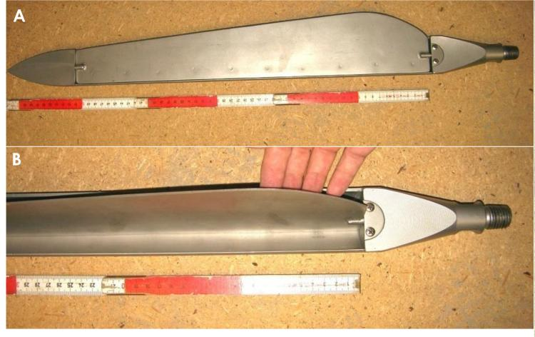
A) and B) Undisturbed peat and lake sediments corers (russian corer); C) coring through the deposits of the Lolair lake (Aosta valley); D) core from lake deposits obtained with a russian corer.
