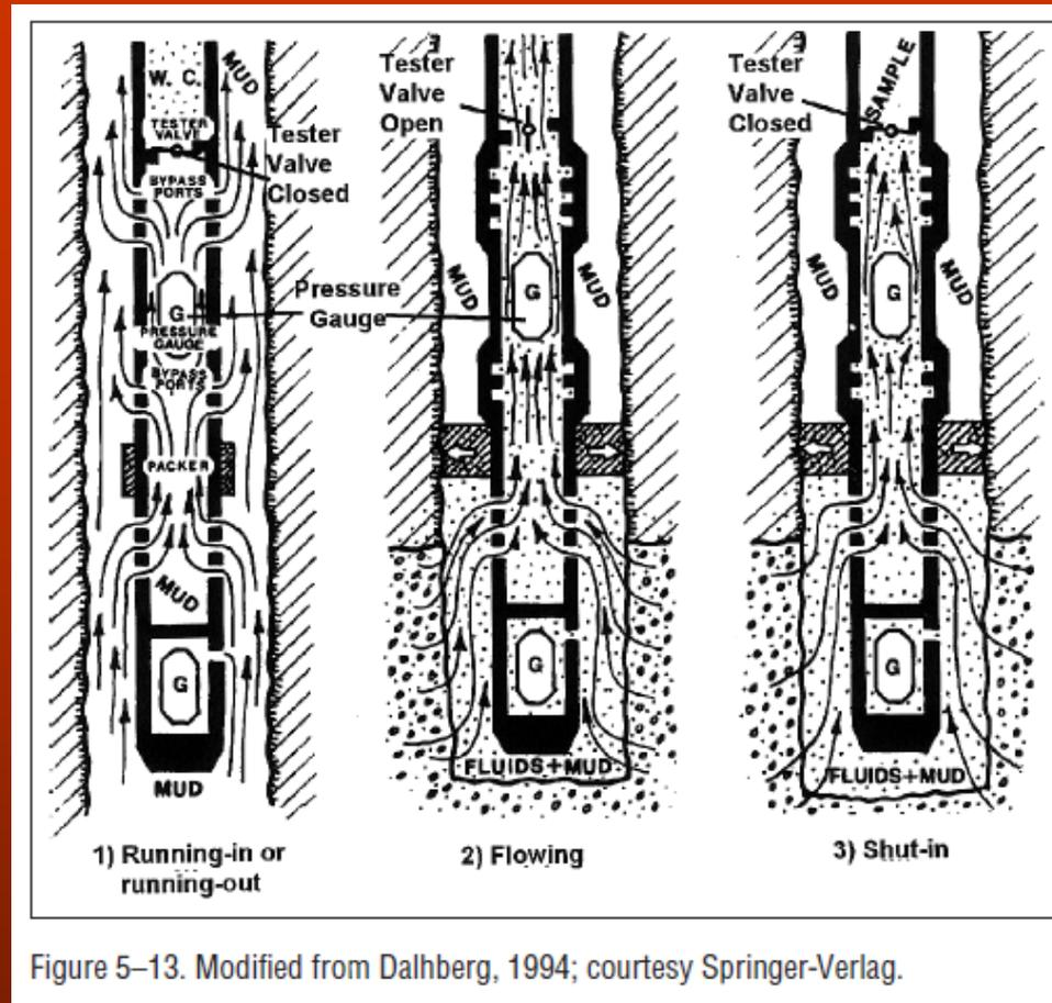
Run in run out period= Tester valve is closed. Drilling fluids flow through the ports
