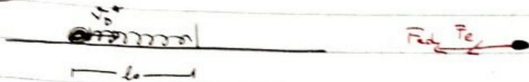
$$-kx - \mu mg = ma \quad \rightarrow \quad a = -\left[\frac{kx}{m} + \mu g\right]$$
