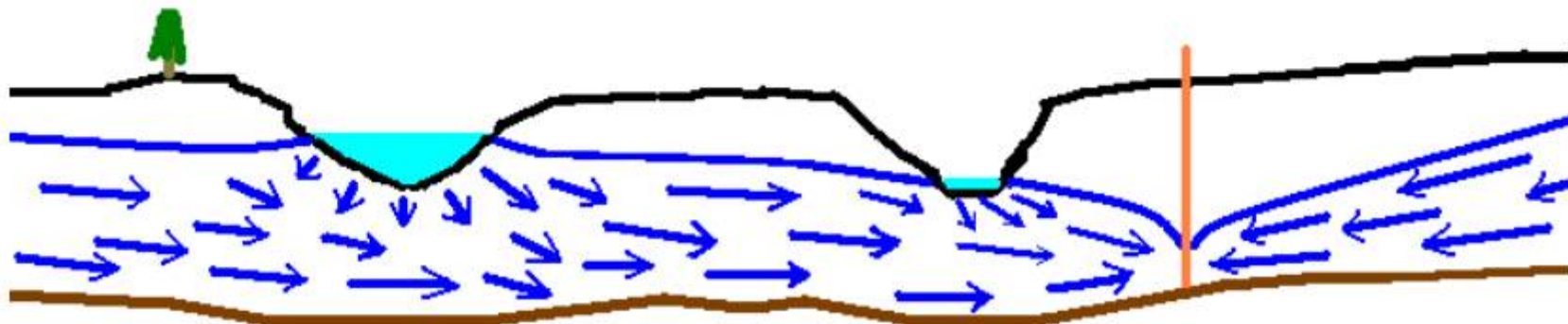
HIGH STREAM FLOW AND AN ACTIVE SUPPLY WELL
