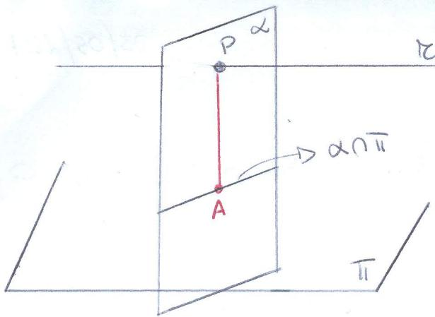
SI PUÒ CALCOLARE  $\overline{PA}$ , DISTANZA TRA  $P$  E  $\alpha \cap \pi'$  NEL PIANO  $\alpha$ .
