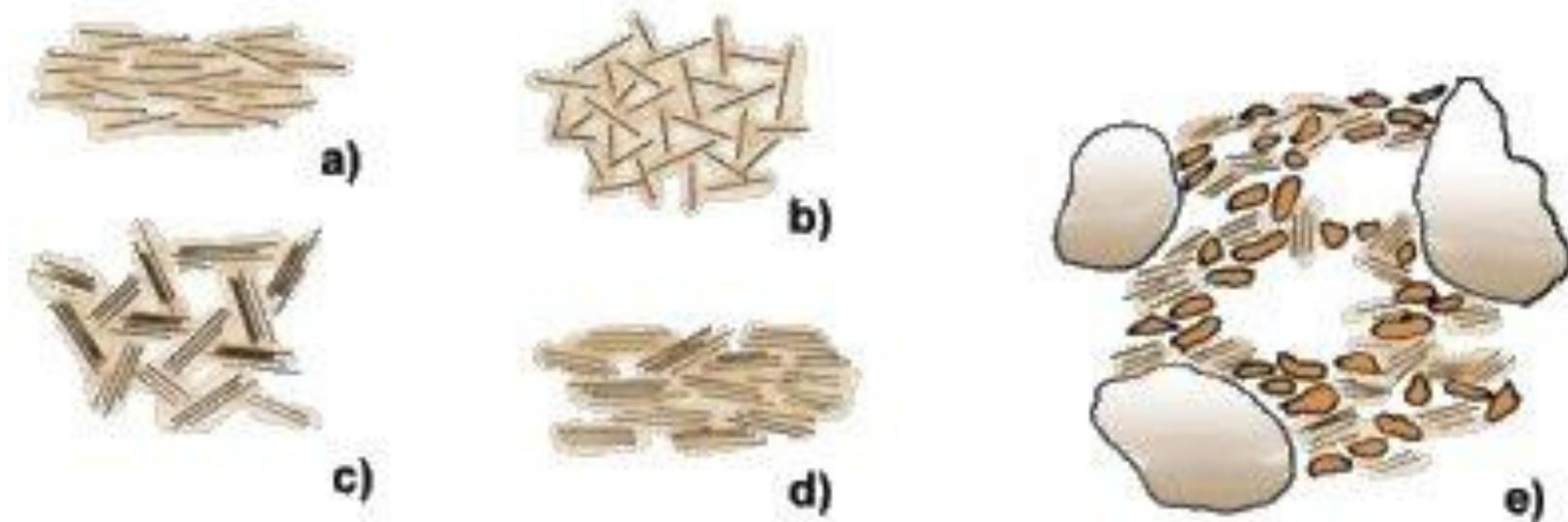
Clay structures: dispersed and oriented (a), flocculated (b), bookhouse (c), turbostratic (d) and the natural structure of clay (after Craig, 1990)
