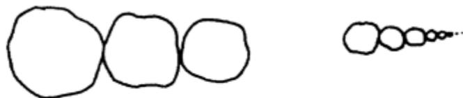
**Figure 4-8. Gap-graded soil.**
