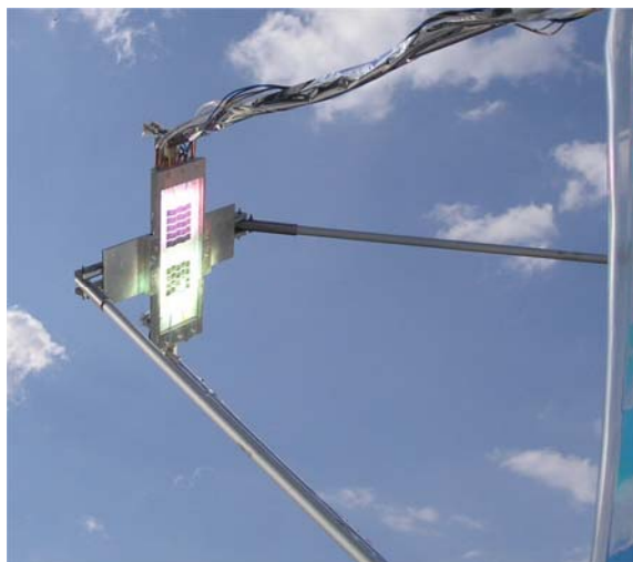
Figure 4-38 – Illuminated receiver in working conditions
