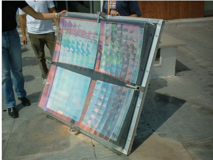
Figure 4-31 – Dichroic flat faceted concentrator with the two shells with films
