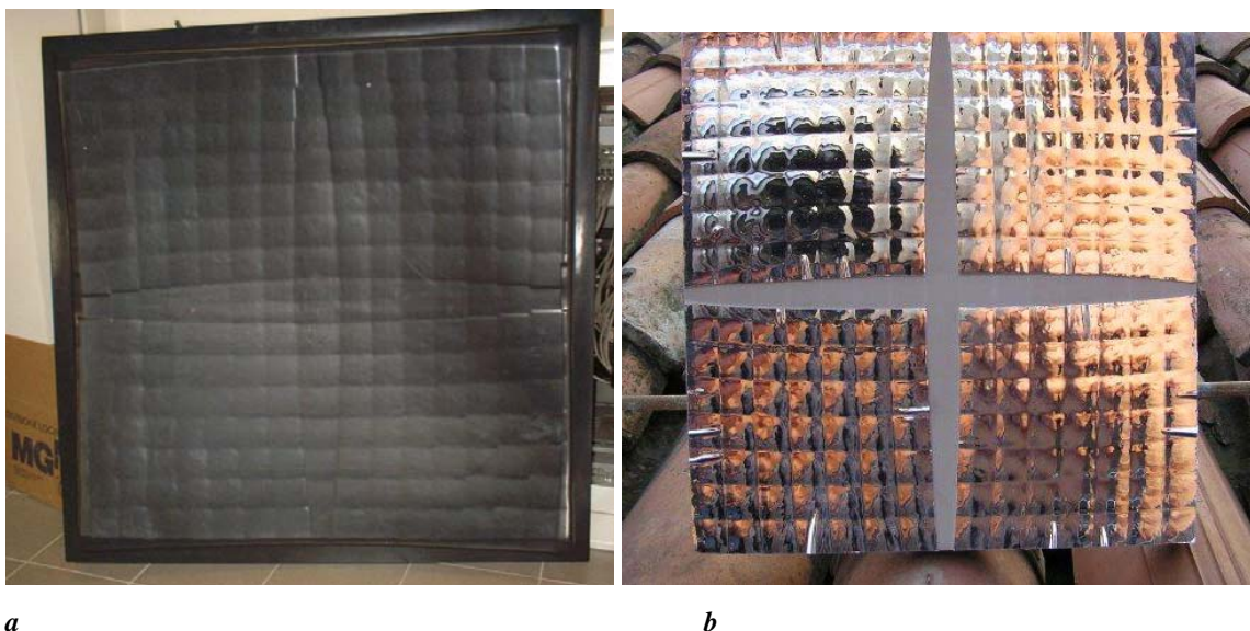
Figure 4-15 – (a) Optimised flat faceted dish in ABS before the reflective cover; (b) small prototype of the dish in (a) with reflective surface
