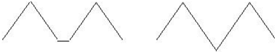
Figure 5-3 – Cross section profile of a non complete etching process and of a finite etching
