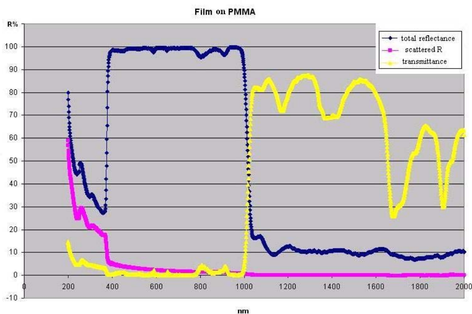
Figure 4-30 - Reflectance and transmittance characteristics for the mirror adhesive film employed
