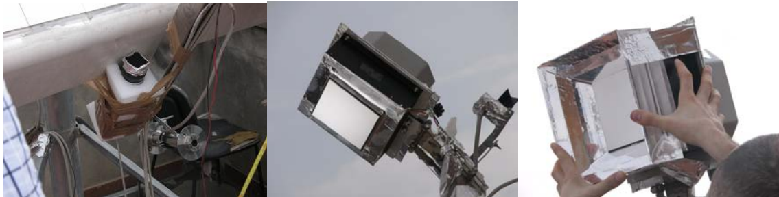
Figure 4-8 – Elements of the experimental set-up for the measurement of flux uniformity of the dish in fig.(4-6b). The CCD camera, the lambertian diffuser and the diffuser with the employed secondary collector are shown.
