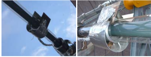
Figure 10: The FVC1 sensor head mounted on the PCS receiver during a test campaign.
