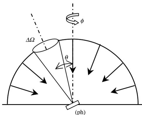
Fig. 1. Illustration of the measurement of irradiance from a diffuse light source. The photodetector (ph) is oriented towards the front hemisphere, by varying angles  $\theta$  and  $\phi$ , and collects light within the solid angle  $\Delta\Omega$ . If the measured irradiance is constant, also the radiance of the source is constant.
