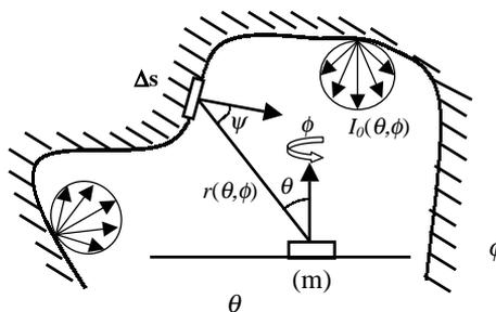
Fig. 3. Illuminated wall surrounding the sample (m). If the light intensity reflected by the wall is homogeneous, i.e. if  $I_0(\theta, \phi) = \text{const.}$ , then the wall behaves like an ideal (lambertian) source of diffuse light.
