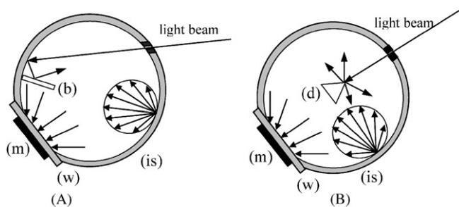
Fig. 4. (A) The sphere (is) is illuminated by a light beam striking its internal wall. (B) The sphere is illuminated by a light beam striking the central diffuser (d). The configuration (b) assures a better homogeneity of light inside the sphere and on the sample (m).
