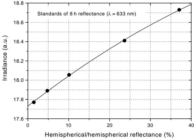
Fig. 5. Example of calibration curve for  $R^{hh}$  measurements. The irradiance measured inside the sphere is reported as function of the reflectance under diffuse light of a set of five standards.
