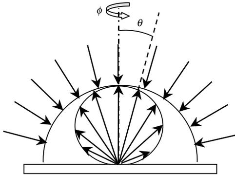
Fig. 2. A source of diffuse light is irradiating the surface of an ideal diffuser (lambertian diffuser). The reflected light is diffused towards the front hemisphere in such a way that its intensity decreases with angle  $\theta$  following a  $\cos \theta$  law, and is independent on the azimuth  $\phi$  (spherical indicatrix).
