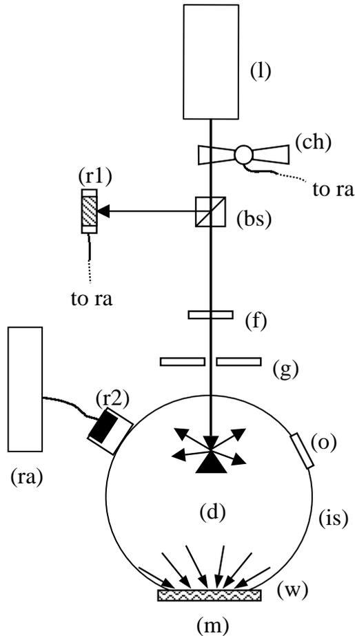
Fig. 6. Schematics of the apparatus HERE used for measurements of  $R^{hh}$  on the PV modules. Components: (l) light source; (ch) mechanical chopper; (bs) beamsplitter; (r1) diode photodetector; (ra) multi-channel radiometer (lock-in); (f) filter; (g) diaphragm; (r2) pyroelectric detector; (o) view port; (d) diffuser; (is) integrating sphere; (w) test window; (m) PV module.
