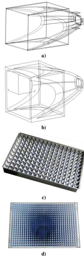
**Figure 4.** a) CAD view of the boxed Rondine<sup>®</sup> Gen1. b) CAD view of the boxed Rondine<sup>®</sup> Gen2. c) Photo of the Rondine Gen 1 CPV module (Wp: =95 W; Eff.: = 12% C = 20X). d) Photo of the Rondine Gen 2 CPV module (Wp: = 120 W; Eff.: = 16% C = 20X)
