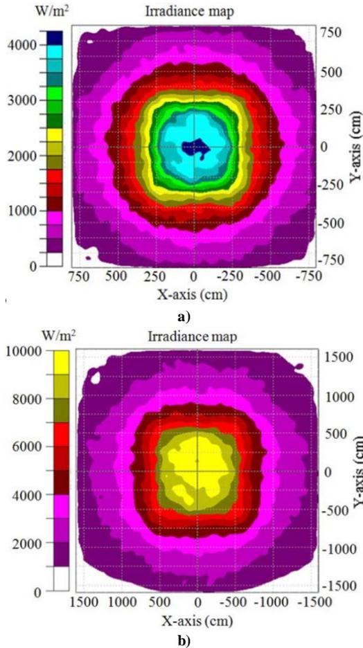
**Figure 10.** Rondine® Gen2: a) flux distribution recorded on the screen (ps) for the P-method; b) flux distribution recorded on the screen (ps) for the PH-method
