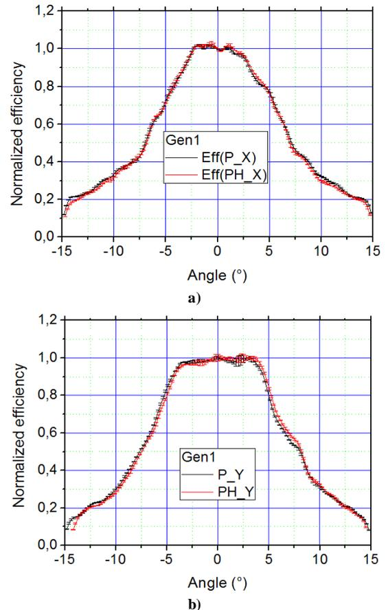
**Figure 9.** Rondine<sup>®</sup> Gen1:  $X$ -axis (a) and  $y$ -axis (b) of the normalized optical efficiency profiles derived by the P-method and the PH-method
