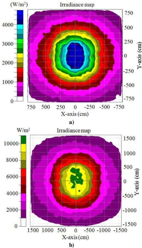
**Figure 8.** Rondine<sup>®</sup> Gen1: a) flux distribution recorded on the screen (ps) for the P-method; b) flux distribution recorded on the screen (ps) for the PH-method
