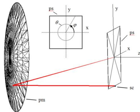
**Figure 3.** Schematic principle of the Parretta-Herrero (PH) method used for simulating the optical properties of a generic solar concentrator. Rays exiting from different points of (sc) at the same polar angle  $\theta$  and azimuthal angle  $\varphi$ , converge on the same point on the screen[31,32]
