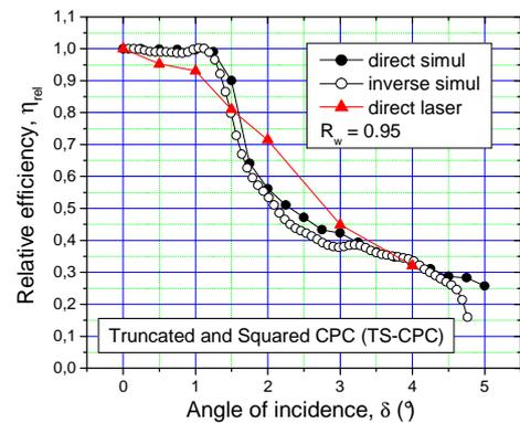
**Figure 7:** Relative optical efficiency  $\eta_{rel}(\delta)$  of TS-CPC obtained by the direct method (dark circles) and the inverse method (white circles).
