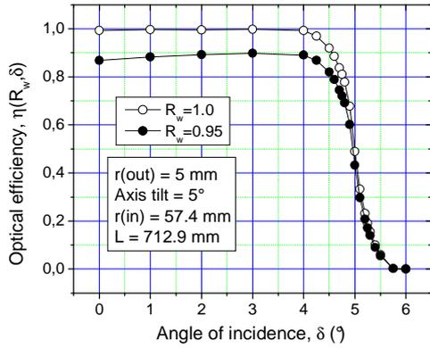
**Figure 2:** Absolute optical efficiency (transmittance) curves obtained by raytracing an ideal 3D-CPC concentrator with 5° acceptance angle, at wall reflectivities  $R_w=1.0$  and 0.95.
