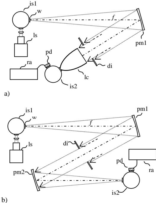
**Figure 1:** a) Schematic of the “direct” method experimental setup for measuring the flux collected by the concentrator (lc) at different angles of incidence. b) Reference setup for measuring the input flux.
