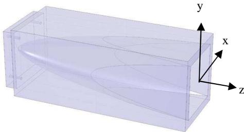
**Figure 5:** CAD image of the TS-CPC concentrator.
