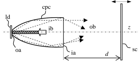
**Figure 3:** Schematic principle of the inverse illumination method (ILLUME).
