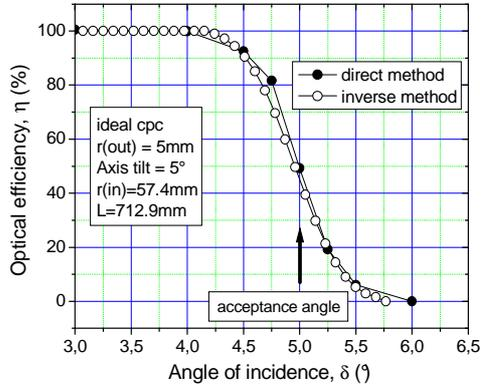
**Figure 4:** Optical efficiency curves of an ideal CPC, calculated by following both the direct (black circles) and the inverse (white circles) illumination method.
