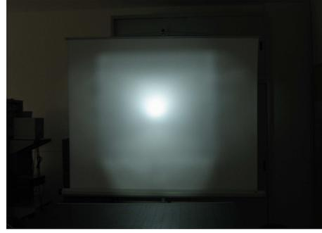
**Figure 9:** Irradiance CCD image of light diffused on the screen (sc) by the TS-CPC illuminated in the inverse mode (ILLUME).
