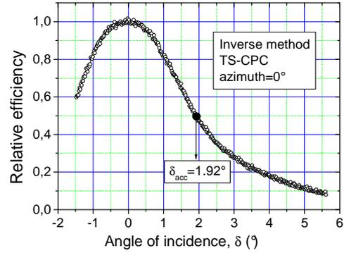
**Figure 10:** Relative radiance profile  $I_{rel}(\delta)$ , calculated applying Eq. (3) to the relative irradiance  $E_{rel}(d, x)$  measured on the screen surface. The radiance profile corresponds to the relative efficiency  $\eta_{rel}(\delta)$  of the CPC concentrator.
