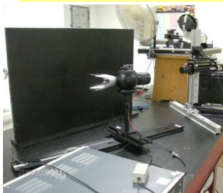
The Rondine is coupled to an integrating sphere
