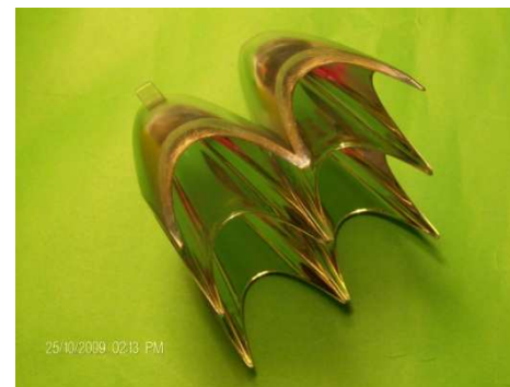
Rondine nonimaging Concentrator (Gen2)
