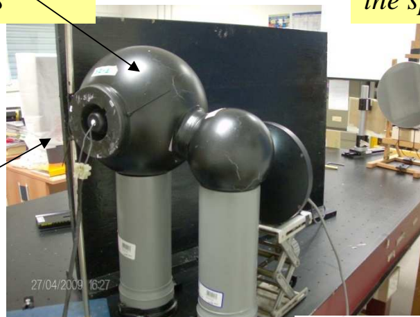
A lamp is placed inside the big sphere
