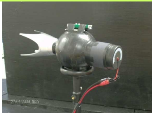
A photodetector is placed inside the integrating sphere
