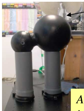
The source: two coupled integrating spheres
