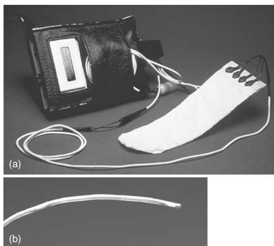
Fig. 49.18 Ambulatory urodynamic equipment demonstrating the (a) digital recording unit, and urilos pad and (b) microtip pressure transducer.
