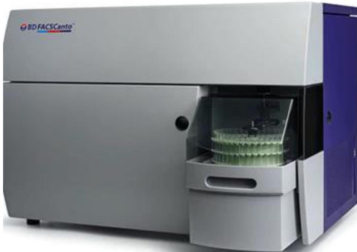
The optics of the BD FACSCanto system consist of an excitation source with three lasers: blue (488-nm, air-cooled, 20-mW solid state), red (640-nm, 40-mW solid state), and violet (405-nm, 30-mW solid state) with a 10 color assay capability
