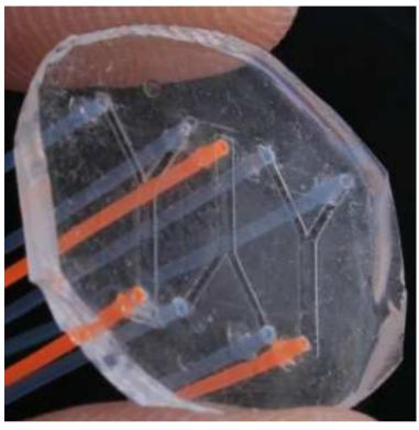
microchannels: 80  $\mu m$  depth, 1.4 cm lenght, 400  $\mu m$  width
