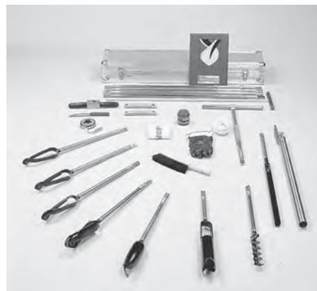
Fig 20 Hand auger with gouge head (second from right) followed by (from right to left) a screw head (suitable for dense soils and sediments), two heads for stony soils, and four heads for general use on fine soils and sediments. (Photograph by Van Walt Ltd)
