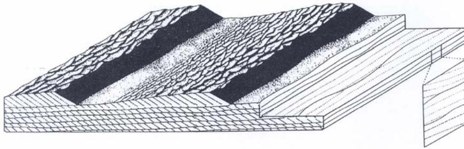
**Figure 3-20** Block diagram of cross-stratification produced by almost perfectly two-dimensional dunes in unidirectional flows
