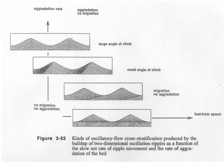
**Figure 3-22** Kinds of oscillatory-flow cross-stratification produced by the buildup of two-dimensional oscillation ripples as a function of the slow net rate of ripple movement and the rate of aggradation of the bed
