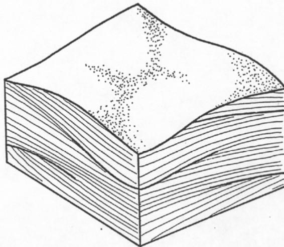
**Figure 3-23** Block diagram of one of the common styles of cross-stratification that's been called hummocky cross-stratification
