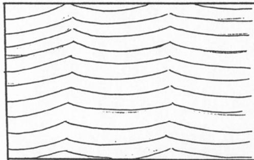
**Figure 3-21** cross-stratification produced by vertical climb of symmetrical oscillation ripples
