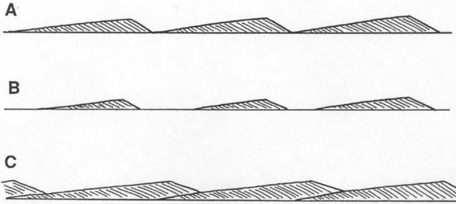
**Figure 3-25** Single-ripple-train cross-stratification. A: full single train. B: starved train. C: ripples starting to overlap.
