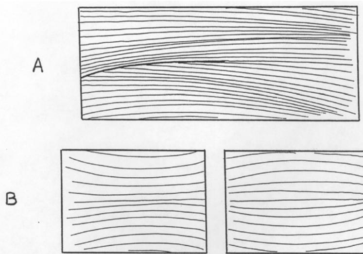
**Figure 3-24** Characteristic small-scale features of the geometry of stratification in hummocky cross-stratification formed by bed aggradation during maintenance of oscillatory-flow bed forms. A: fanning of truncation surfaces laterally into conformable sequences of laminae. B: tendency for convex-up sets of laminae to be succeeded upward by concave-up sets, and vice-versa
