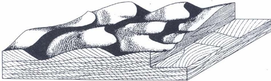
**Figure 3-19** Block diagram of cross-stratification produced by three-dimensional dunes in unidirectional flows
