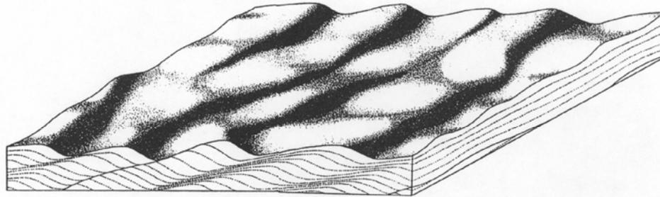
**Figure 3-18** Block diagram showing geometry of climbing-ripple cross-stratification produced at large angles of climb
