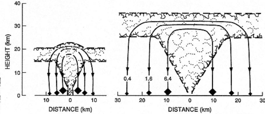
Clast trajectories from the umbrella region of a Plinian eruption column; clast sizes are given in centimeters. Note that the dispersal is greater for the 35-km-high column than for the 21-km-high column. (Adapted from Carey and Sparks, 1986.)
