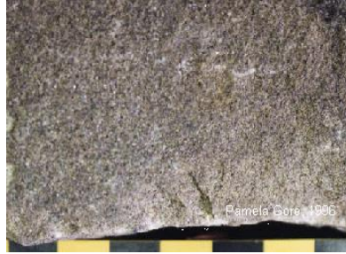
Grains visible with naked eye (course), with aid of x10 hand lens (fine)
