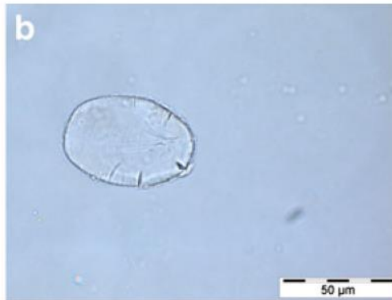
Damaged starch granule (17 µm diameter) viewed under polarized light (SD 1327i)
