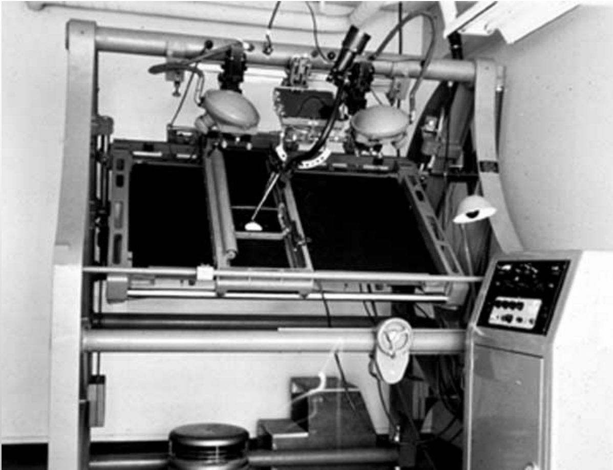
Photograph of the T-64 orthophotoscope, designed and built in 1964 by Russell Bean at USGS Headquarters in Virginia
