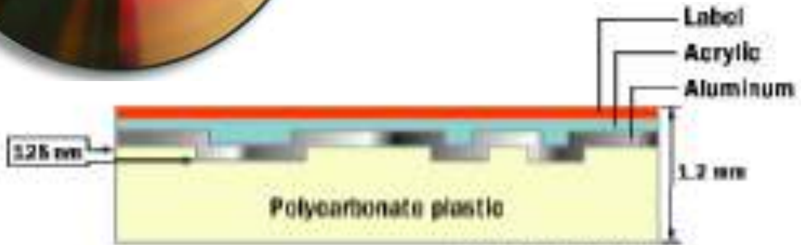
©2000 HowStuffWorks Cross-section of a CD
