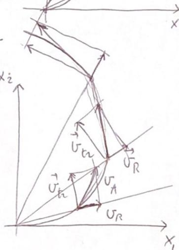
$$\vec{a}_A = \underbrace{\vec{a}_R}_0 + \underbrace{\vec{a}_{tr}}_{\vec{\omega} \times \vec{v}_R} + \underbrace{\vec{a}_{co}}$$
