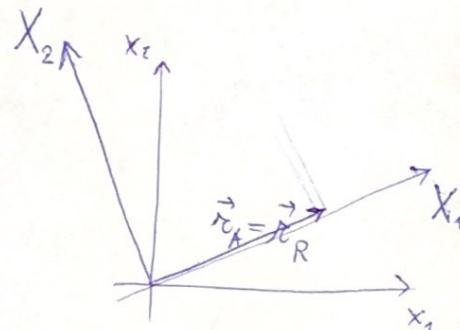
$$\vec{a}_A = \underbrace{\vec{a}_R}_{0} + \vec{a}_{tr} + \vec{a}_n$$
