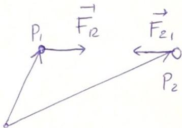
$$\begin{aligned}\vec{M}_{012} &= \vec{OP}_1 \times \vec{F}_{12} \\ \vec{M}_{021} &= \vec{OP}_2 \times \vec{F}_{21}\end{aligned}$$
