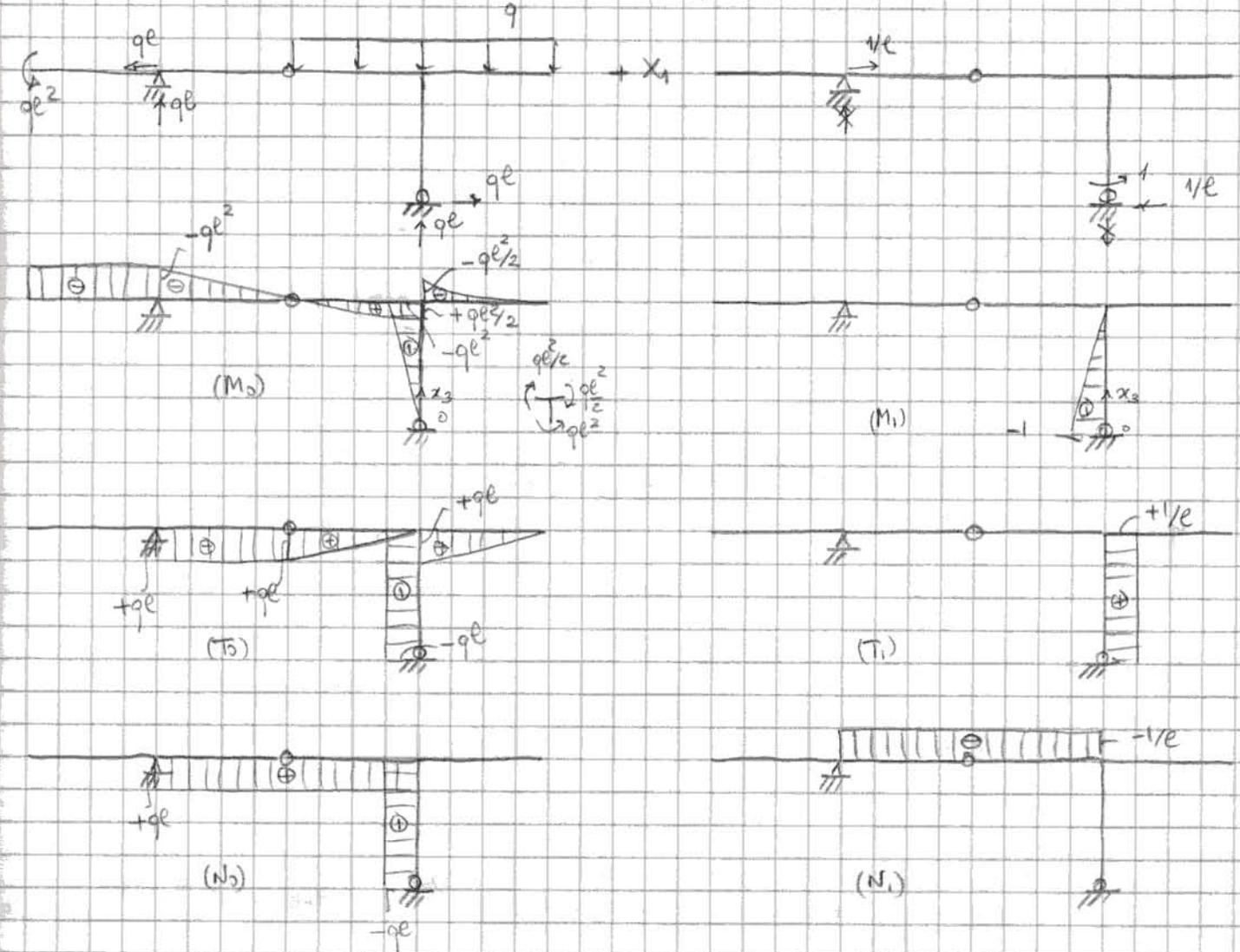
$$EI \eta_{10} = \int_0^e (-qe^2 x_3) \left(-1 + \frac{x_3}{e}\right) dx_3 = -qe^2 \int_0^e \left[-x_3 + \frac{x_3^2}{e}\right] = -qe^2 \left[-\frac{e^2}{2} + \frac{e^3}{3e}\right] = \frac{qe^3}{6}$$
