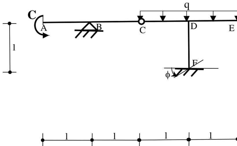
$$l = 1 \text{ m}, q = 1 \text{ t/m}, C = ql^2, \sigma_{AMM} = 2400 \text{ kg/cm}^2$$
