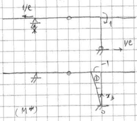
$$\begin{aligned} 1. \varphi_D &= \frac{1}{EI_1} \int_0^l \left( -\frac{x_3}{l} \right) \left( \frac{ql^2}{2} - \frac{3}{2} qlx_3 \right) dx_3 \\ &= \frac{1}{EI_1} \int_0^l \left[ \frac{3}{2} qx_3^2 - \frac{qlx_3}{2} \right] dx_3 \\ &= \frac{1}{EI_1} \left[ \frac{q}{2} l^3 - \frac{ql^3}{4} \right] = \frac{ql^3}{4EI_1} = \frac{10 \cdot 100^3}{4 \cdot 2,1 \cdot 10^6 \cdot 318} = 0,91^\circ \end{aligned}$$
