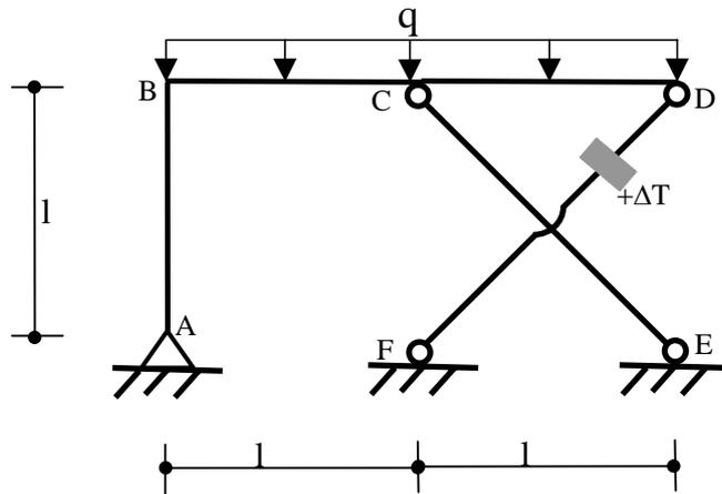
$$l = 1.5 \text{ m}, q = 2 \text{ t/m}, \sigma_{AMM} = 2400 \text{ kg/cm}^2$$
