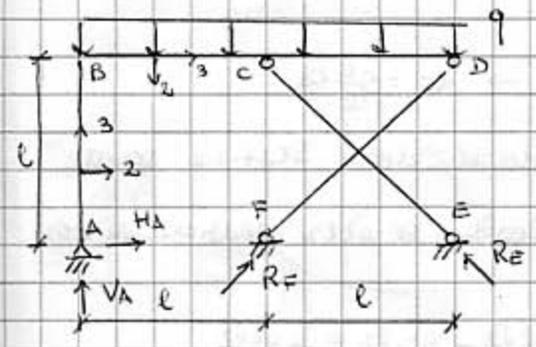
$$\begin{aligned} (\rightarrow) \quad H_A + R_F \frac{\sqrt{2}}{2} - R_E \frac{\sqrt{2}}{2} &= 0 \\ (\uparrow) \quad V_A + R_F \frac{\sqrt{2}}{2} + R_E \frac{\sqrt{2}}{2} &= 2ql \\ (A\uparrow) \quad R_F \frac{\sqrt{2}}{2} l + R_E \frac{\sqrt{2}}{2} 2l &= 2ql^2 \end{aligned}$$
