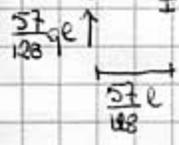
$R_F = q l \frac{\sqrt{2}}{2} + \frac{7}{128} q l^2 \frac{\sqrt{2}}{l} = \frac{\sqrt{2}}{2} q l \left( 1 + \frac{7}{64} \right) = \frac{71 \sqrt{2}}{128} q l = 2354 \text{ kg}$
