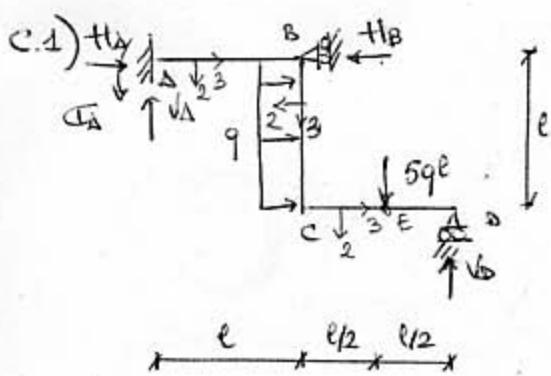
$$\begin{aligned} & \text{(1)} \quad H_A = H_B - qe \\ & \text{(2)} \quad V_A + V_B = 5qe \\ & \text{(3)} \quad M_A + V_B 2e = \frac{5qe}{2} \cdot \frac{3e}{2} - \frac{qe^2}{2} \end{aligned}$$
