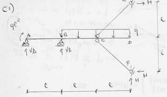
$$\begin{aligned} (\uparrow) \quad V_A + V_B + 2H &= 2qe \\ (\curvearrowright) \quad V_B 2e + V_B e &= -qe^2 \end{aligned}$$
