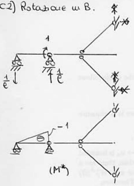
$$1 \cdot \varphi_B = \frac{1}{EI_1} \int_0^l \left(-\frac{x_3}{l}\right) \left(q l^2 - \frac{19}{16} q l x_3\right) dx_3$$
