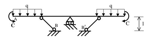
$$\begin{split} 1 &= 1 \text{ m, } q = 20 \text{ kN/m, } C = 20 \text{ kNm} \\ E &= 210 \text{ GPa, } \sigma_{\text{AMM}} = 240 \text{ MPa} \end{split}$$
