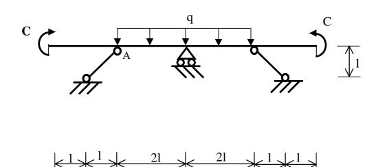
$$l = 1 \text{ m}, q = 25 \text{ kN/m}, C = 25 \text{ kNm}$$
