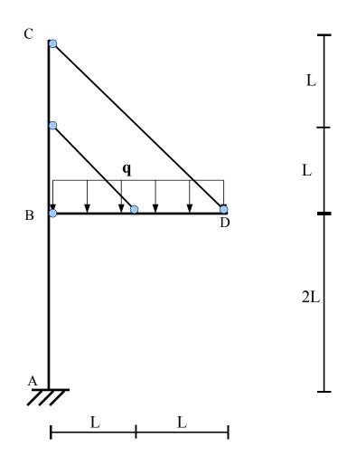
$$L = 2 \text{ m, } q = 20 \text{ kN/m,}$$
