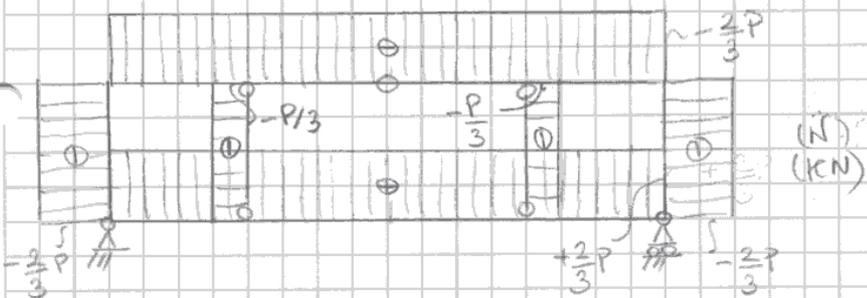
Dimensionamento:  $W_1 \geq \frac{2}{3} \frac{PL}{\sigma_{adm}} = \frac{2}{3} \frac{50 \cdot 10^3}{240 \cdot 10^8} = 1,38 \cdot 10^{-4} \text{ m} = 138 \text{ cm}^3$
