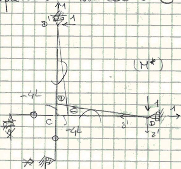
$$\begin{aligned} \delta \cdot v_D &= \frac{1}{EI_1} \int_0^{4L} (-x_{z1}') \left(-q \frac{x_{z1}'^2}{2}\right) dx_{z1}' \\ &= \frac{1}{EI_1} \frac{q}{2} \left[ \frac{x_{z1}'^3}{3} \right]_0^{4L} \\ &= \frac{1}{EI_1} \frac{q \cdot 256}{8} = \frac{32qL^4}{EI_1} \\ &= \frac{32 \cdot 20 \cdot 10^3 \cdot 10^2}{210 \cdot 10^9 \cdot 11770 \cdot 10^{-8}} \text{ cm} \\ &= 2,6 \text{ cm} \end{aligned}$$
