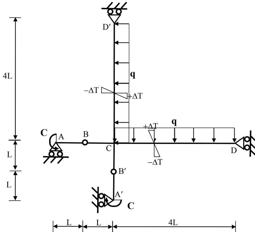
$$L = 1 \text{ m}, q = 20 \text{ kN/m}, C = 40 \text{ kN m}$$
