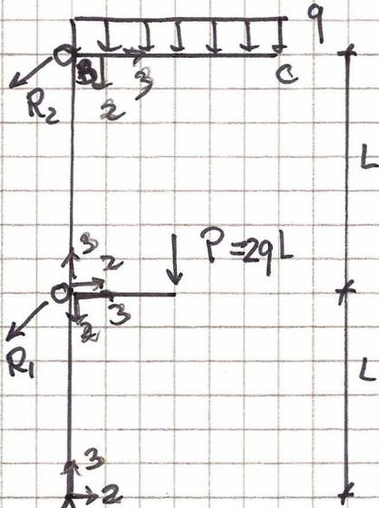
$$\begin{aligned} (\rightarrow) R_1 \frac{\sqrt{2}}{2} + R_2 \frac{\sqrt{2}}{2} &= 0 \\ \rightarrow R_1 &= -R_2 \end{aligned}$$
