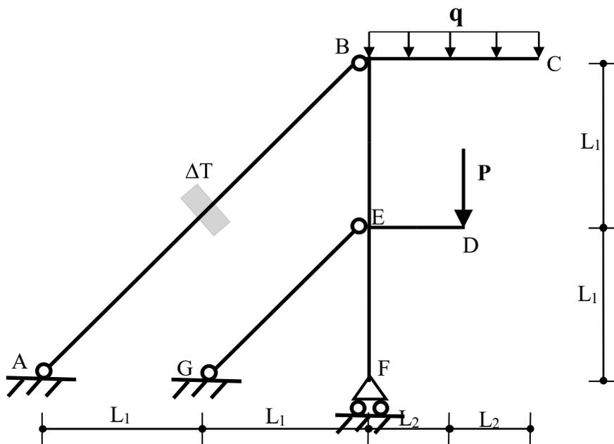
$$L_1 = 1 \text{ m}, L_2 = 0.5 \text{ m}, q = 20 \text{ kN/m}, P = 40 \text{ kN}$$
