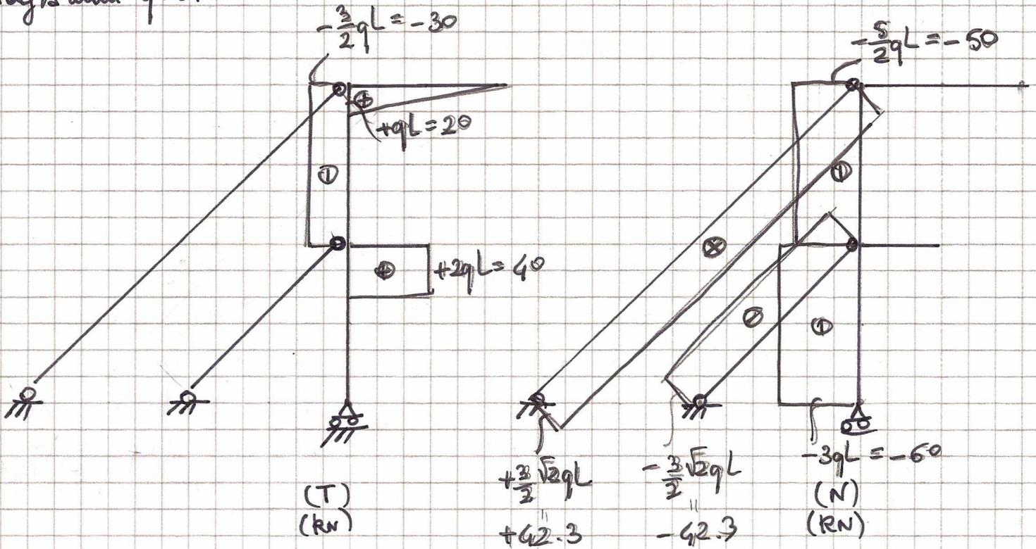
Progetto:  $W_1 \geq \frac{M_{max}}{\sigma_{amm}} = \frac{qL^2}{8\sigma_{amm}} = \frac{20 \cdot 10^3 \text{ Nm}^2}{8 \cdot 210 \cdot 10^6 \text{ N}} = \frac{1}{12} \frac{10^6 \text{ cm}^3}{10^8} = 83.3 \text{ cm}^3$
