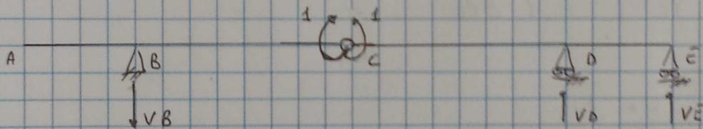
$$\curvearrowright \text{CBA} \quad V_B \cdot 2L = 1 \quad \underline{V_B = \frac{1}{2L}}$$
