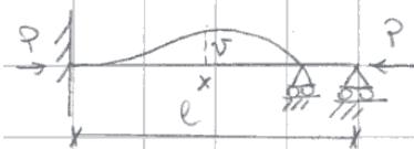
Free-body diagram: •  $V, C$  reactions at the built-in end (they do not depend upon  $x$ ).
