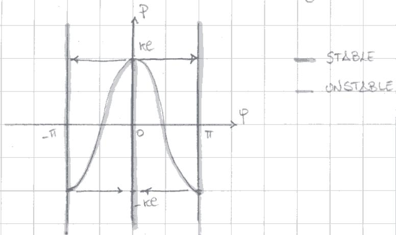
REM: These structures are characterized by the absence of deformation before reaching the critical load, which coincides with bifurcation load. The stability analysis of these structures falls into the class of Eulerian problems.
