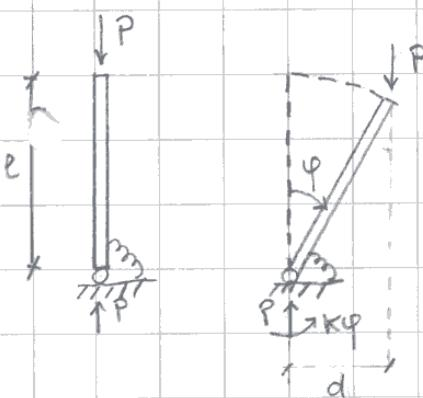
Consider a rigid beam of length  $l$  subject to a compressive dead load of intensity  $P$  applied to its free end. The other extremity is constrained by a hinge connected to a rotational spring (torsion spring) of elastic constant  $K$  [Nm] obeying a linear law:
