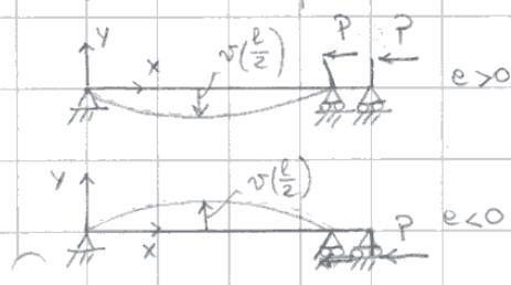
The values of  $v\left(\frac{l}{2}\right)$  increase non-linearly with increasing  $P$ . At  $P = P_{cr}$  an infinitely large value of  $v$  occurs but material breakdown occurs at some smaller value of  $P$ .
