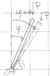
Imagine to perturb the equilibrium, i.e. to vary the equilibrium configuration  $\varphi$ , solution to (1), of an angle  $\alpha$ .
