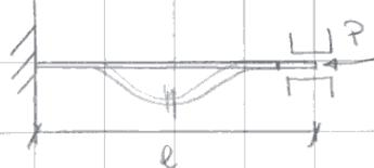
$$P_{cr} = \frac{\pi^2 EI}{(l/2)^2} \quad \text{"doubled Euler's strut"} \\ \text{equivalent length } L = l/2$$
