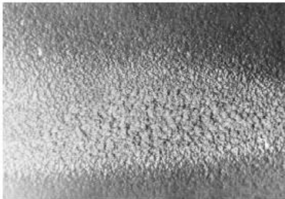
Figure 34 Cavitation on the leading edge, suction side of a runner Maha, Pankaj Das, Acharya. Bureau of Reclamation photo.
