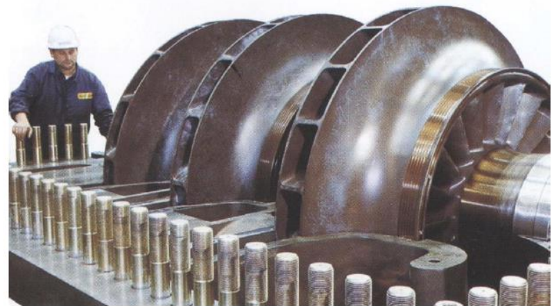
GE Centrifugal compressor
