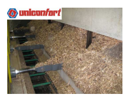
Figure 3.29 Sliding bar conveyor used for the discharge of bunkers Explanations: 1 = hydraulic generator, 2 = bearing for hydraulic cylinder, 3 = hydraulic cylinder, 4 = sliding bars, 5 = control screw, 6 = drop channel, 7 = screw conveyor, 8 = delivery end.
