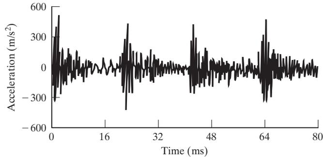
**FIGURE 10.38** Time-domain waveform of a faulty gearbox [10.23].
