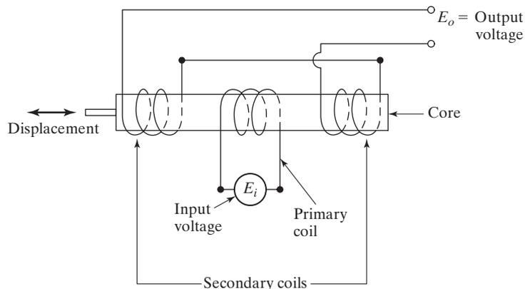
FIGURE 10.7 Schematic diagram of an LVDT transducer.
