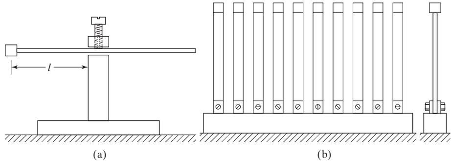
FIGURE 10.15 Frequency-measuring instruments.
