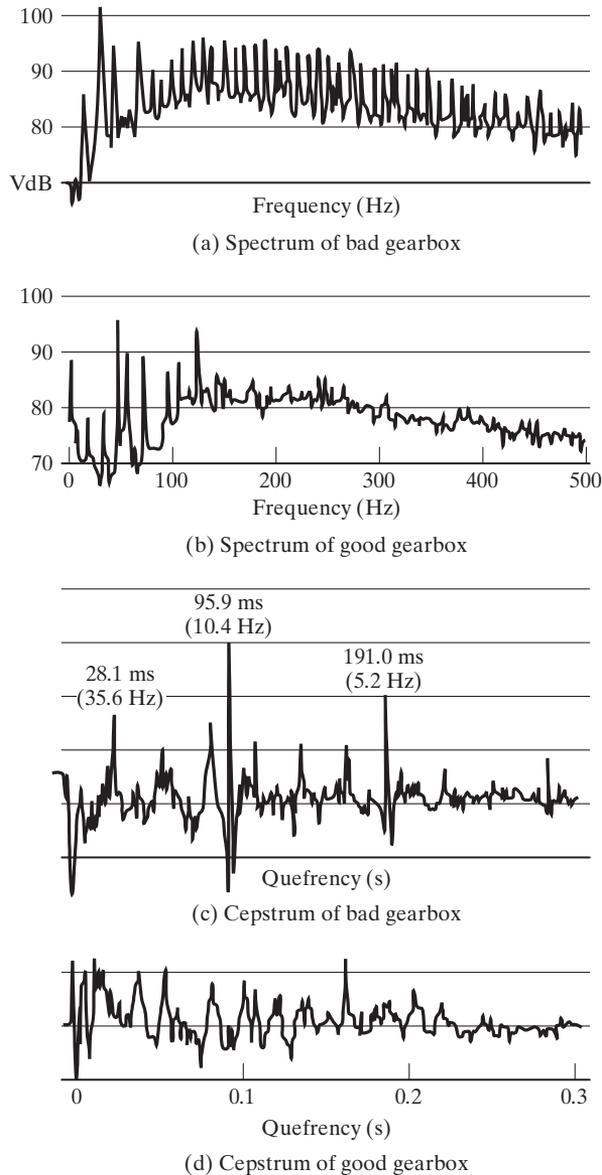
**FIGURE 10.41** Spectrum and cepstrum of a gearbox [10.24].
