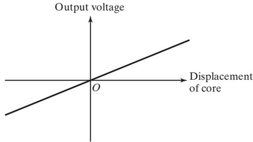
**FIGURE 10.8** Linearity of voltage with displacement of core.
