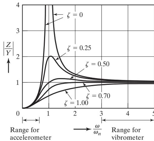
**FIGURE 10.10** Response of a vibration-measuring instrument.
