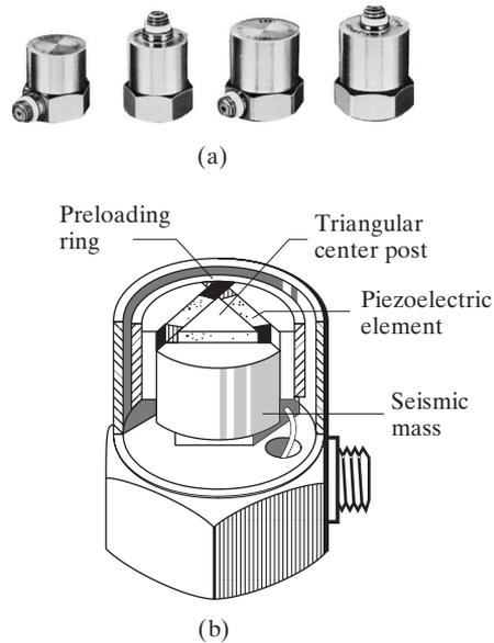
**FIGURE 10.12** Accelerometers.
