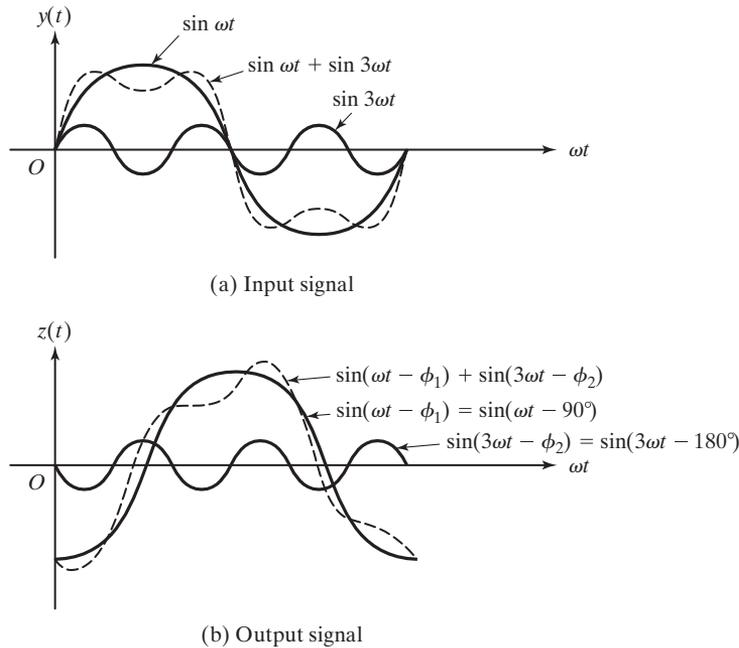
FIGURE 10.14 Phase-shift error.
