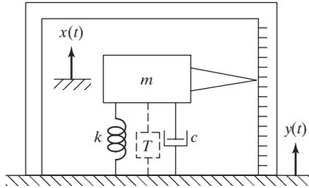
**FIGURE 10.9** Seismic instrument.
