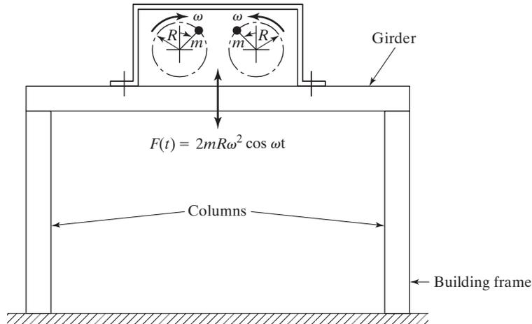
FIGURE 10.18 Vibration excitation due to unbalanced force.
