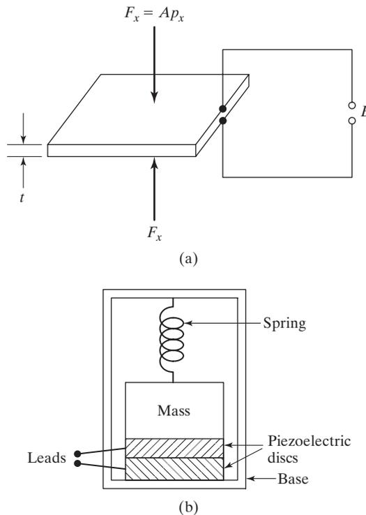
FIGURE 10.5 Piezoelectric accelerometer.
