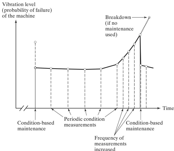
FIGURE 10.35 Condition-based maintenance.
