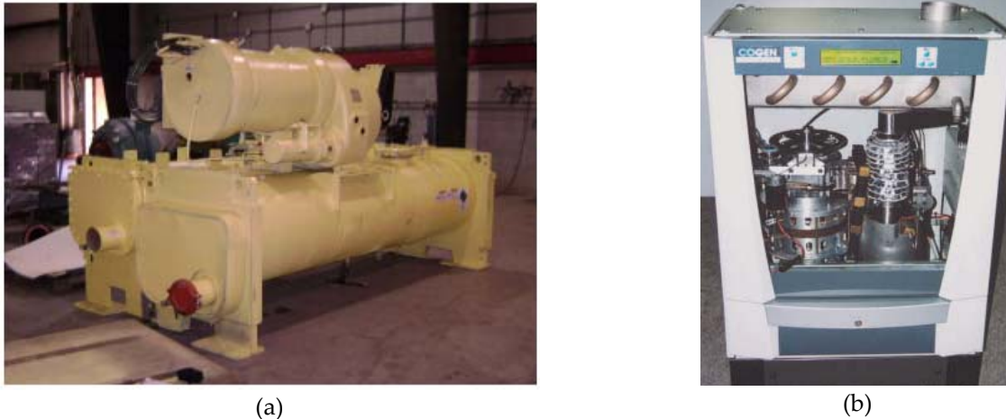
Fig. 2.2.3.1 - MCR (a) Infinity da 50 kW e (b) Cogen Microsystems da 2.5 kW
