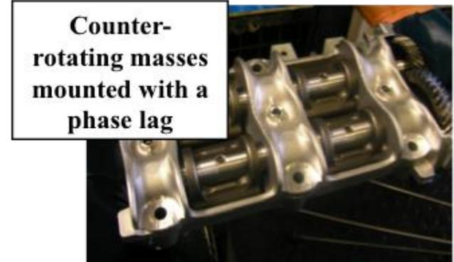
**Counter-rotating masses mounted with a phase lag**
