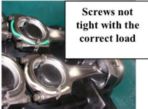
**Screws not tight with the correct load**
