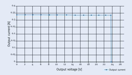
High accurate current/ voltage regulation using TLE 4305G and CoolSETTM ICE B0365JG
