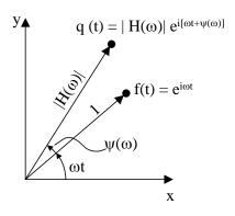
$$\begin{split} f(t) &= e^{i\omega t} \Rightarrow \qquad q(t) = \left| H(\omega) \right| e^{i\left[\omega t + \psi(\omega)\right]} \\ \left| H(\omega) \right| &= \frac{1}{m \omega_0^2} \frac{1}{\sqrt{\left(1 - \frac{\omega^2}{\omega_0^2}\right)^2 + 4\xi^2 \frac{\omega^2}{\omega_0^2}}} \\ \psi(\omega) &= \arctan\left\{ -\frac{2\xi \frac{\omega}{\omega_0}}{1 - \frac{\omega^2}{\omega_0^2}} \right\} \end{split}$$
