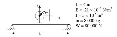
$$K = \frac{48EJ}{L^3} = 7875000 \text{ N/m} \Rightarrow q_S = \text{W/K} = 0.01 \text{ m}$$
