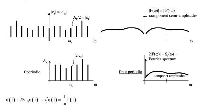
The steady-state response q(t) to a generic force f(t) can be expressed as the integral of the elementary component responses to the elementary component harmonic forces:
