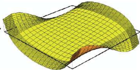
Shear force  $v_y$  (7.73 versus 12.1 kN/m). Thickness is 2,250 mm
