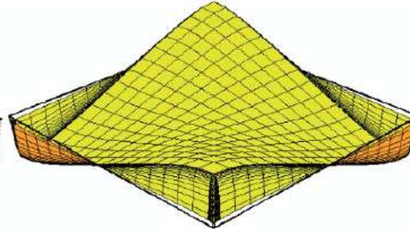
Torsion moments  $m_{xy}$  (9.69 versus 9.39 kNm/m). Thickness 200 mm
