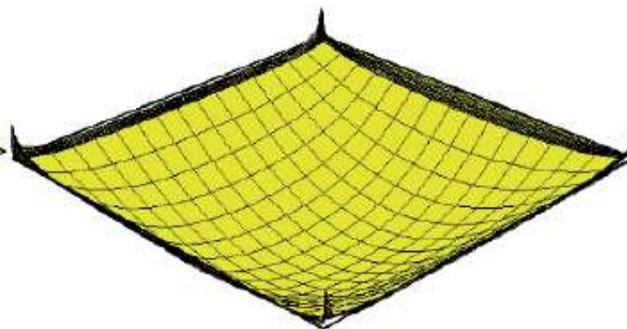
Bending moment  $m_x$  (-10.1 versus -10.3 kNm/m) Thickness is 200 mm
