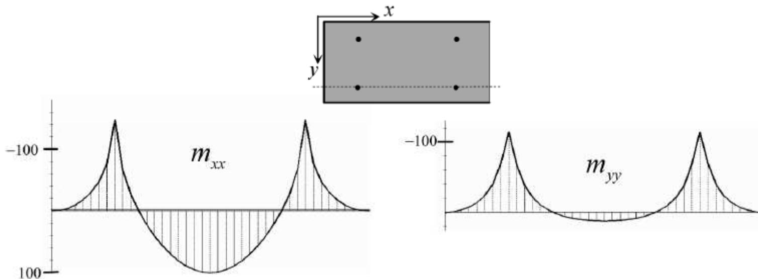
**Figure 14.3** Moment diagrams in section over columns.
