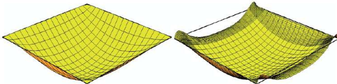
Bending moment  $m_{xx}$  (10.2 versus 11.9 kNm/m). Thickness is 2,250 mm
