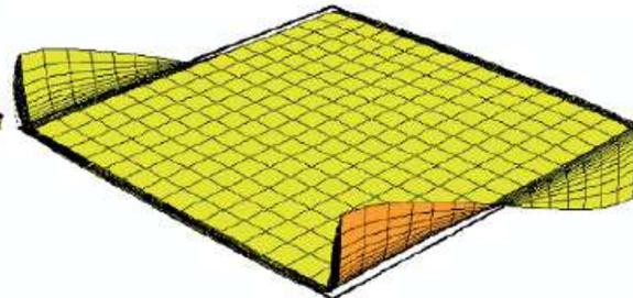
Shear force  $v_x$  (8.77 versus 11.53 kN/m). Thickness 200 mm
