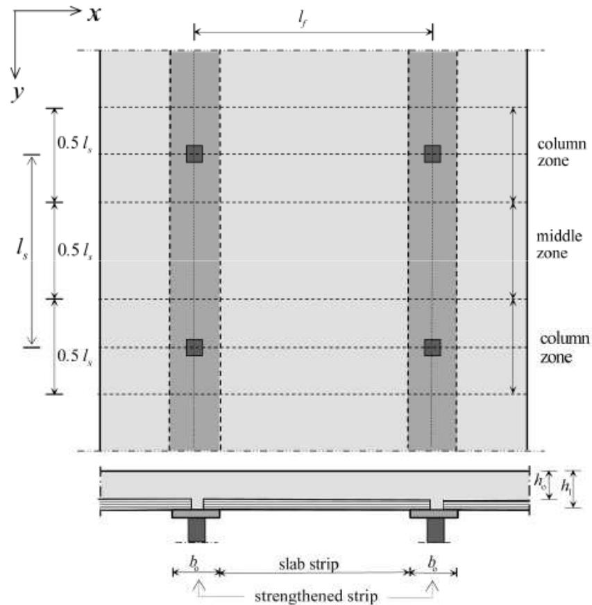
Figure 17.9 Strengthened strips over columns.
