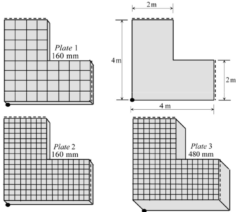
Figure 15.1 Three plates. Mesh fineness and thickness varied.
