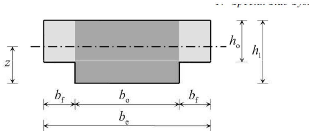
**Figure 17.10** Effective width of strengthened strip.
