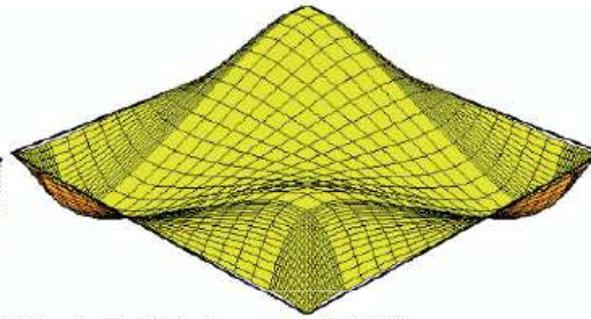
Twisting moments  $m_{xy}$  (9.28 versus 6.87 kNm/m). Thickness is 2,250 mm
