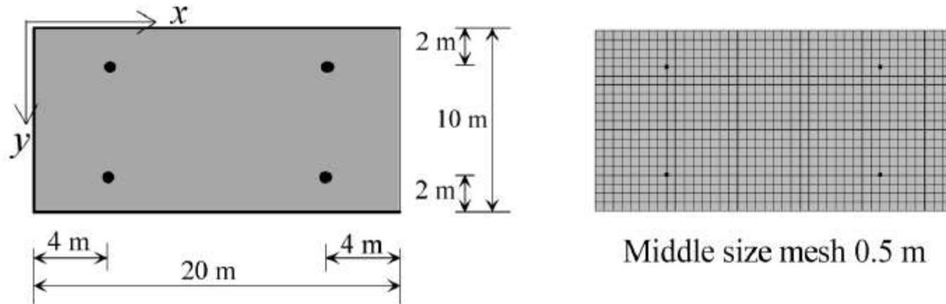
Figure 14.1 Rectangular slab on inward columns.
