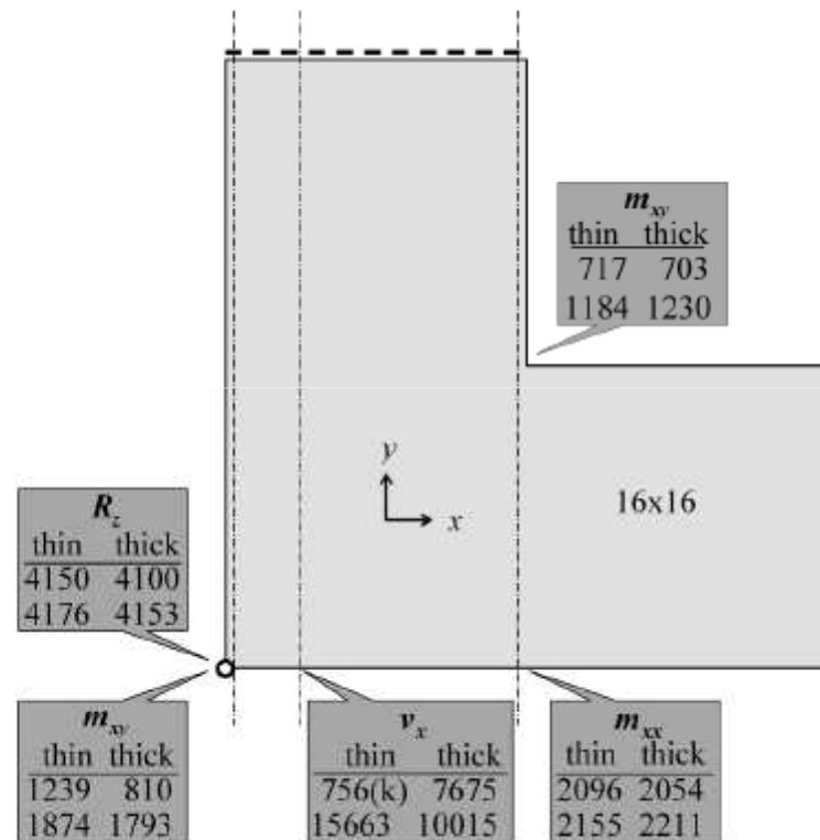
**Figure 15.2** Big scatter in submitted results for twisting moment and shear force.
