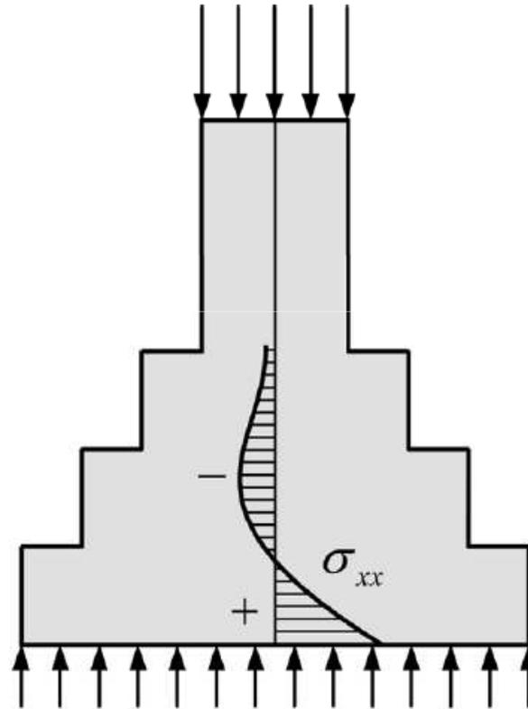
**Figure 2.22** Foundation foot. Stresses and strut-and-tie scheme.
