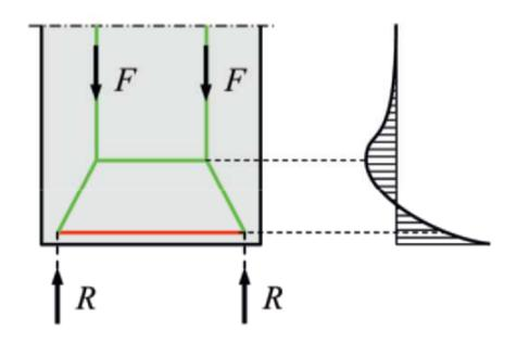
Figure 2.15 Strut-and-tie model for silo wall.
