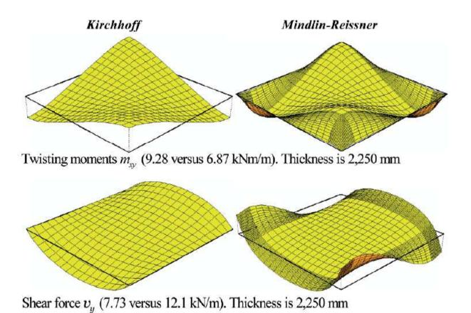
Figure 15.13 Twisting moment and shear force in thick plate.
