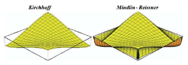
Torsion moments  $m_{xy}$  (9.69 versus 9.39 kNm/m). Thickness 200 mm
