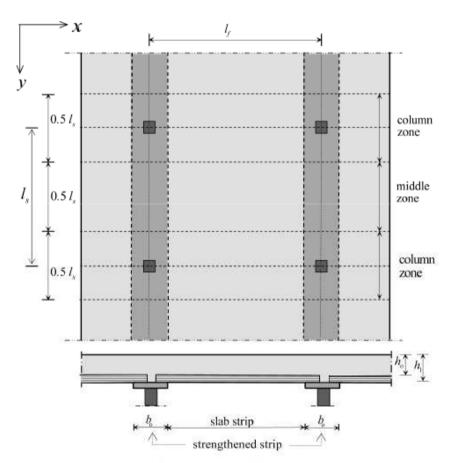
Figure 17.9 Strengthened strips over columns.
