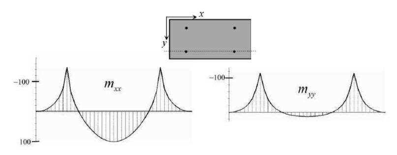
Figure 14.3 Moment diagrams in section over columns.
