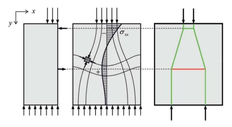
**Figure 2.21** Load spreading (for example the anchorage of a pre-stressed cable in a beam).
