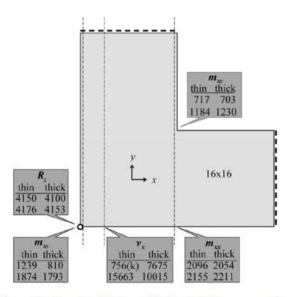
Figure 15.2 Big scatter in submitted results for twisting moment and shear force. Units in N and m.
