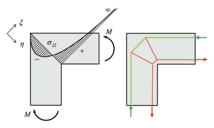
Figure 2.24 Beam-column connection. Stresses and strut-and-tie scheme.
