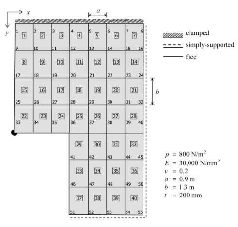
Figure 12.1 Mesh of a plate with node and element numbering.
