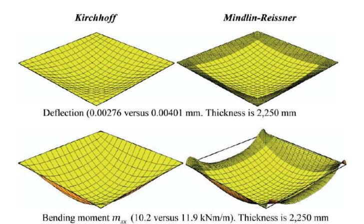
Figure 15.12 Mesh, deflection and bending moment for thick plate.
