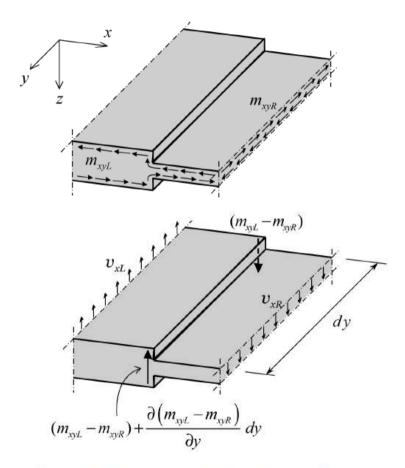
Figure 4.14 Twisting moment at discontinuity in thickness.
