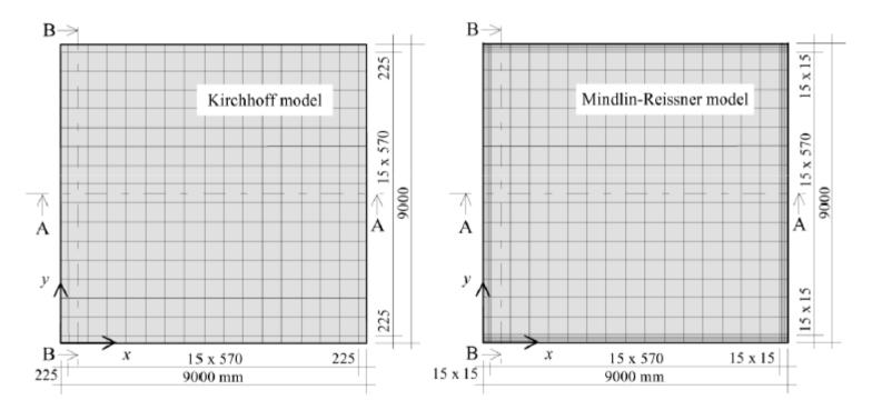
**Figure 15.8** Mesh for thin plate analyses.
