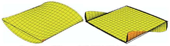
Shear force  $v_x$  (8.77 versus 11.53 kN/m). Thickness 200 mm
