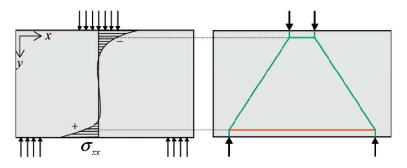
Figure 2.20 Foundation block. Stresses and strut-and-tie scheme.
