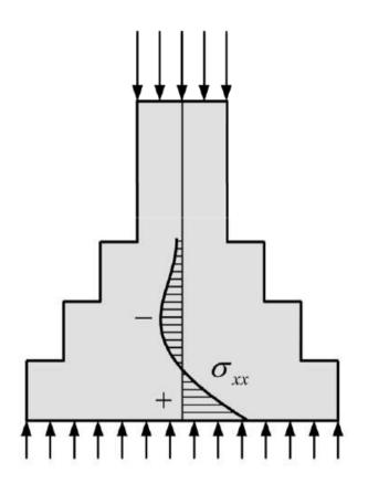
Figure 2.22 Foundation foot. Stresses and strut-and-tie scheme.
