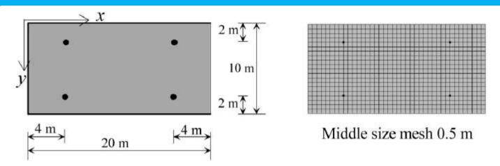
Figure 14.1 Rectangular slab on inward columns.
