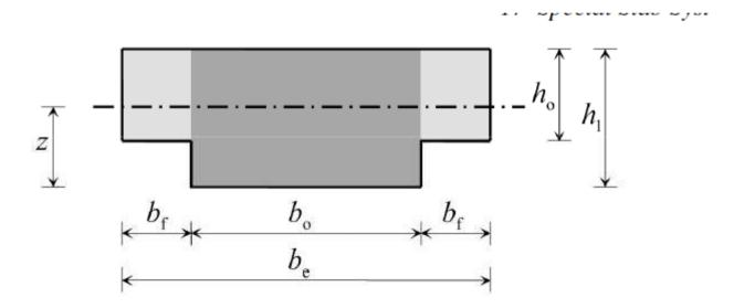
Figure 17.10 Effective width of strengthened strip.
