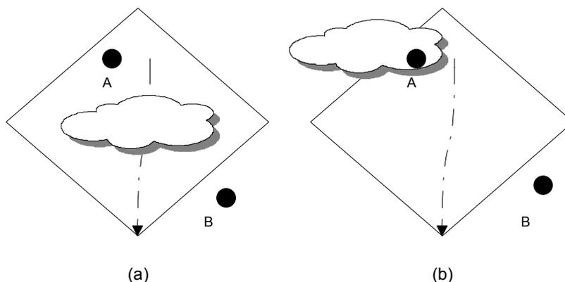
Figure 4-7. Lack of coverage can complicate MAP estimation
