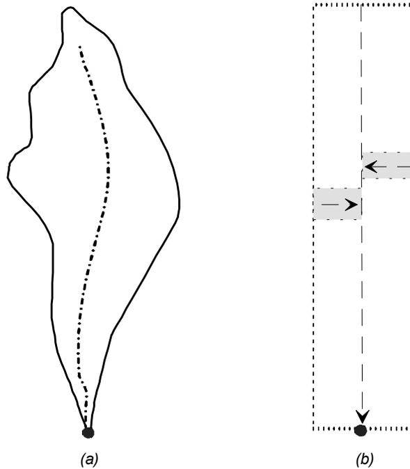
Figure 6-3. Simple watershed with kinematic-wave model representation
