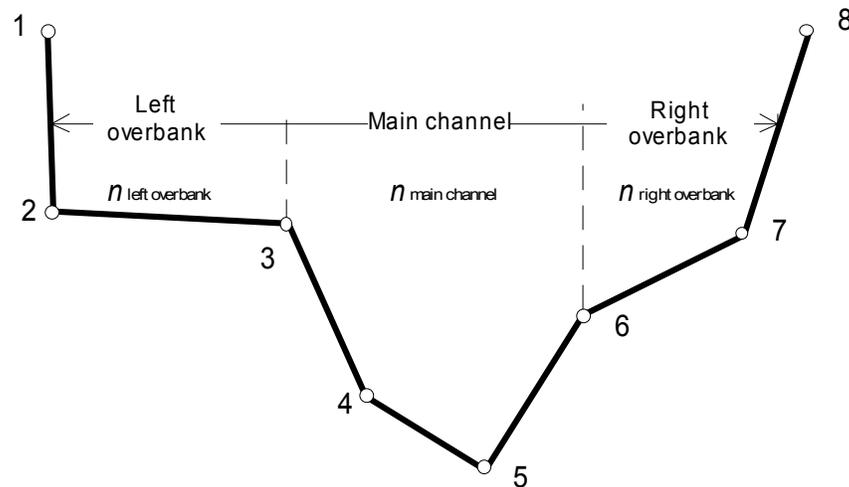
Figure 8-5. Format for describing channel geometry with 8 points
