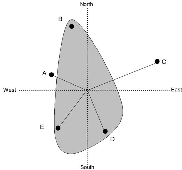
Figure 4-5. Illustration of inverse-distance-squared scheme
