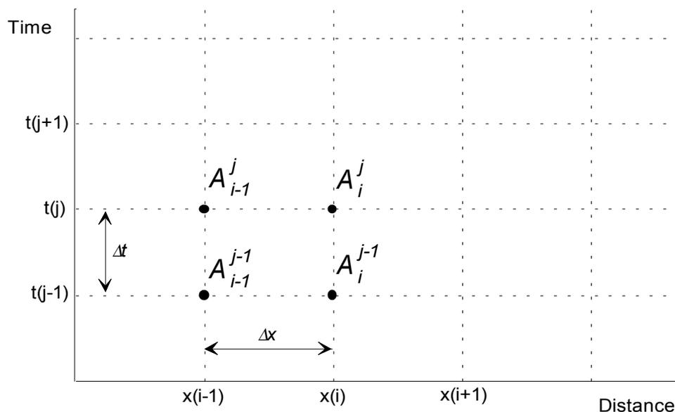
Figure 6-5. Finite difference method space-time grid
