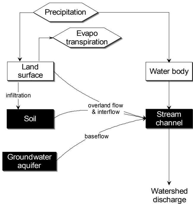
Figure 3-2. Typical HEC-HMS representation of watershed runoff
