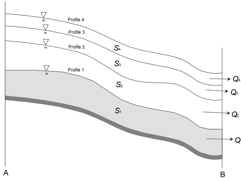
Figure 8-1. Steady-flow water-surface profiles and storage-outflow curve
