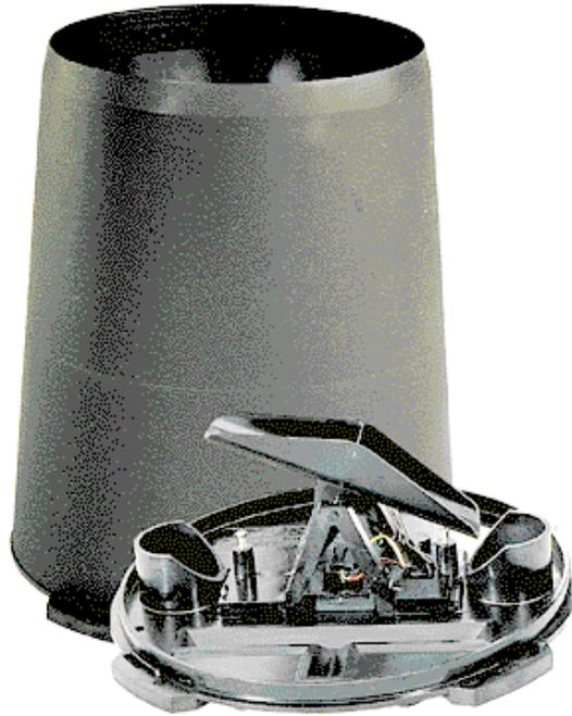
Figure 4-2. Telemetering precipitation observation gage (from www.weathershop.com)
