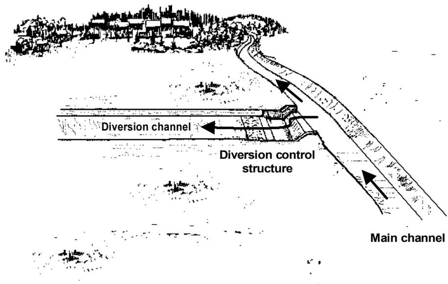
Figure 10-1. Illustration of diversion structure
