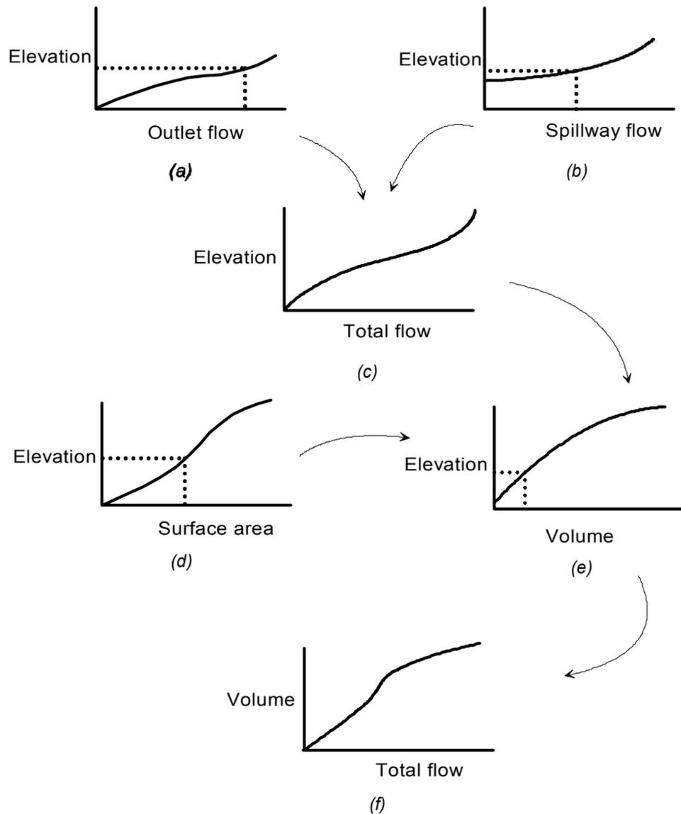
Figure 10-5. Illustration of procedure for defining storage-outflow relationship
