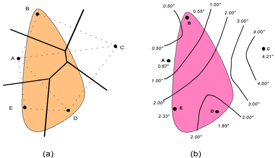
Figure 4-3. Illustration of MAP depth computation schemes
