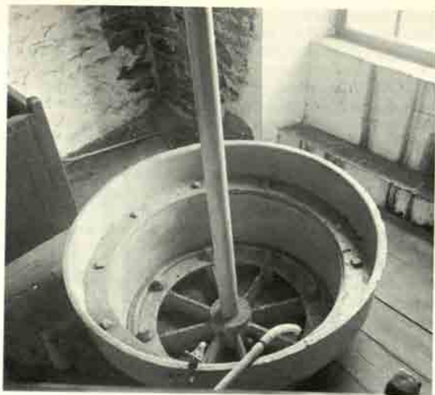
10 Elsecar beam engine. Open top of steam cylinder showing piston
