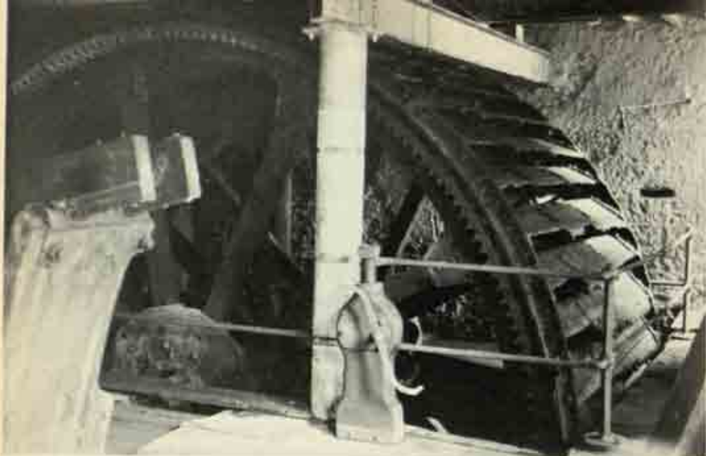
48 Higher Mill, Helmshore, Lancashire. An iron breastshot waterwheel with peripheral gearing and wooden floats
