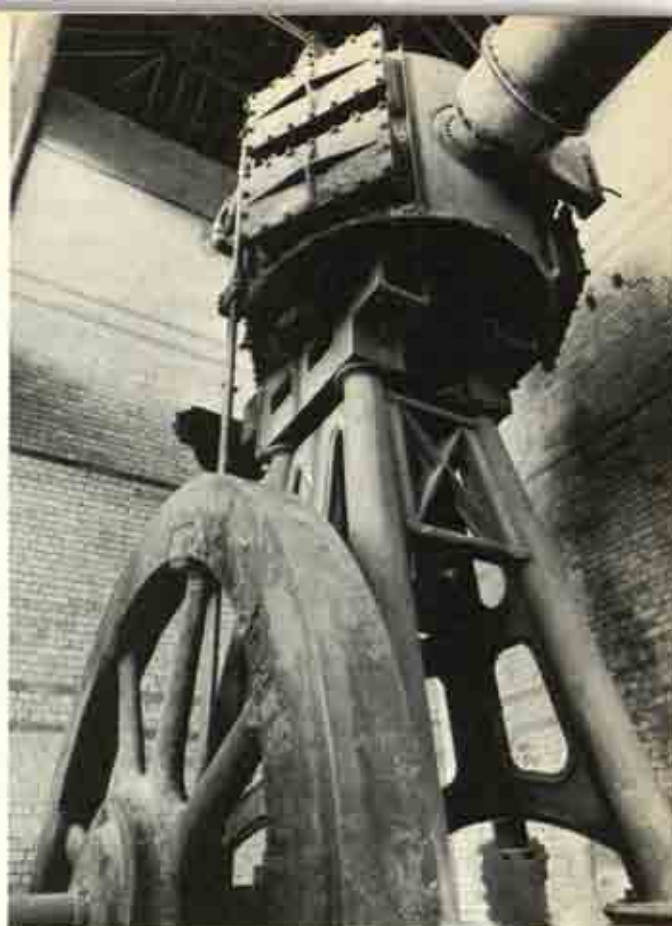
25 Vertical blast-furnace blowing engine, preserved at the Blists Hill Open Air Museum, Ironbridge, Shropshire
