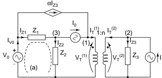
con  $Z_1 = 2 \text{ k}\Omega + 2j \text{ k}\Omega$ ,  $Z_2 = -2j \text{ k}\Omega$ ,  $Z_3 = 2 \text{ k}\Omega - 500j \Omega$ ,  $V_0 = 4 \text{ V}$ ,  $I_0 = 3\sqrt{2}e^{-j\pi/4} \text{ mA} = 3 \text{ mA} - 3j \text{ mA}$ ,  $I_1 = e^{j\pi/2} \text{ mA} = j \text{ mA}$ .
